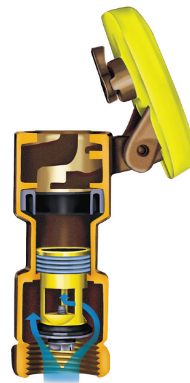
Quick-Coupling Valve Cutaway
